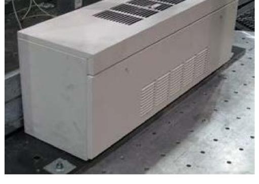
The unit was mounted at the bottom and back using four manufacturer-provided angle clips (one on each front bottom corner and two at the back of the unit at approximately 7 inches high). Each clip was held in place using four #12, 3/4-inch long sheet metal screws; two screws were attached through the unit, and two through the DCL-provided steel fixture.
