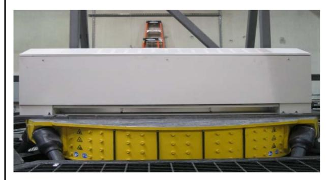
The unit was mounted at the base using four #14 sheet metal screws through the flange at the unit's base. The unit was mounted at the back using the two manufacturer-provided brackets integral to the unit and one 1/2-inch diameter Grade 5 bolt per bracket to attach the unit to the DCL shake table interface frame. The manufacturer-provided brackets at the back of the unit were located at approximately 12 inches from the unit's base.
