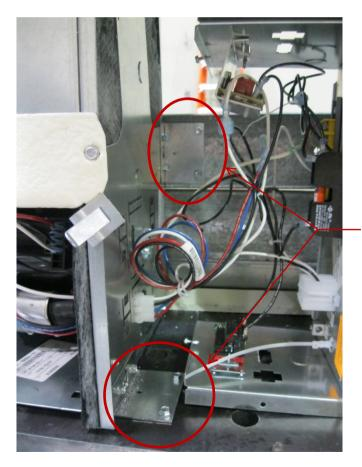
Mounting locations at back and base of unit (interior view of unit)
